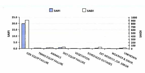
**GEN EQUIP FAILURE** F:83.3% D:82.1% TRANS EQUIP FAILURE F:2.1% D:1.4% ANIMALS F:3.2% D:2.8% DIST EQUIP FAILURE F:3.8% D:4.6% **VEGETATION** F:0.8% D:0.7% **SCHEDULED OUTAGES** F:1.7% D:1 2% EXT INTERFER./OP. ERROR F:2.1% D:4.4% WEATHER & ENVIR. F:0.4% D:0.1% UNKNOWN F:2.4% D:2.7%
