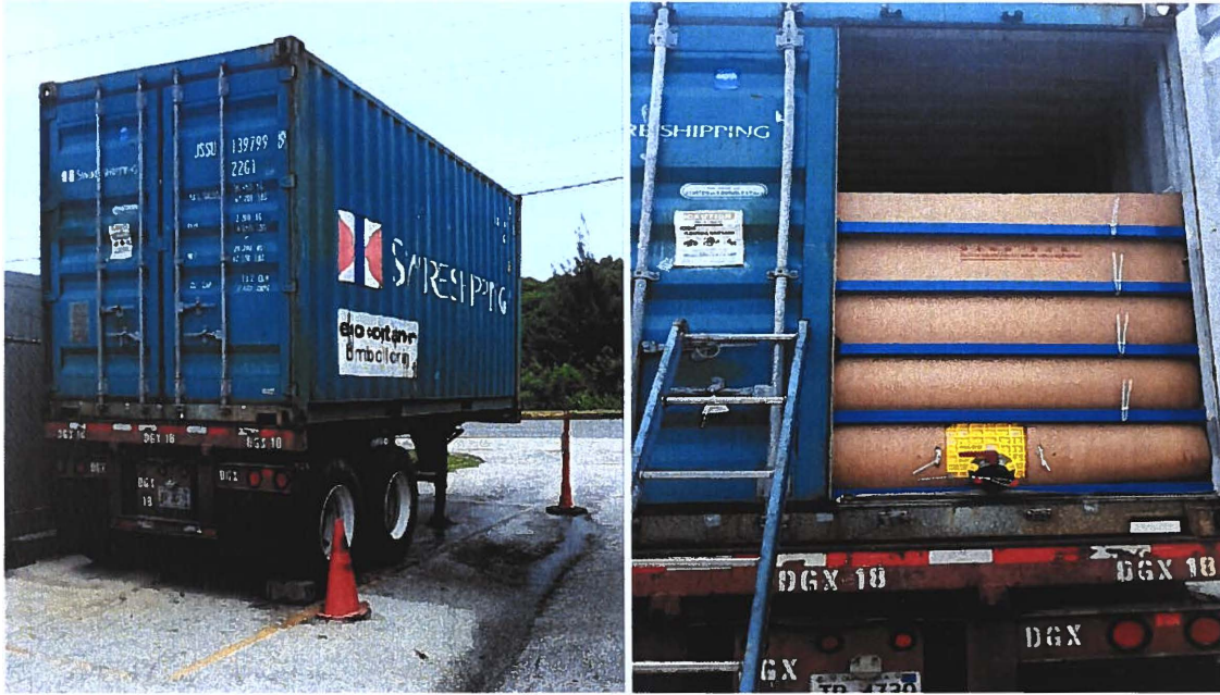
20' DELIVERY CONTAINER WITH UREA BLADDER
