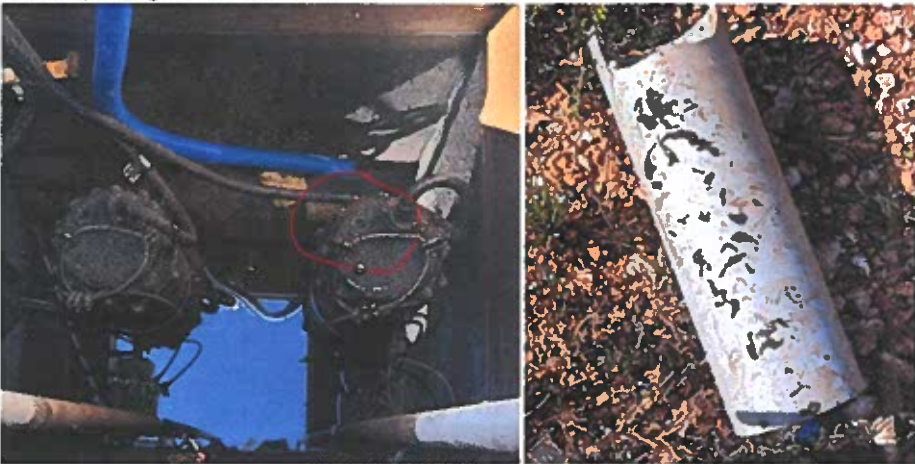
PVC Pipe Fragments in the NDWWTP Reuse Water Pond
